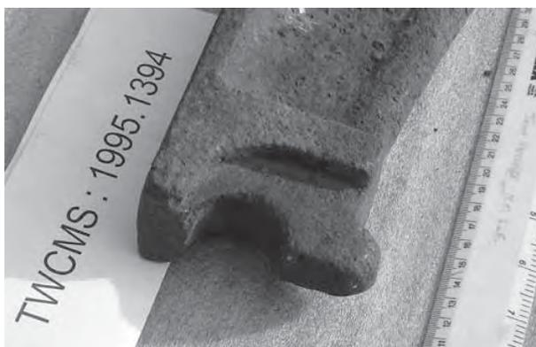
**Figure 8:** Mating joint of fish-belly rail section at the Discovery Museum, Newcastle, UK (Clayson, 2009).
