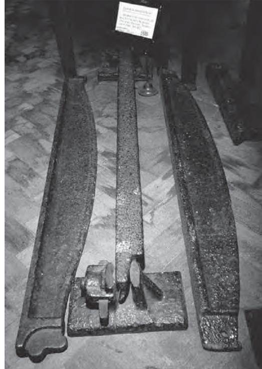
**Figure 7:** 1970 photo of various cast iron rail sections at the Newcastle Discovery Centre. The rail on the left is considered to be very similar to the rail relic found in Newcastle, Australia, in 2004 (Photo: Lewis, 2007).
