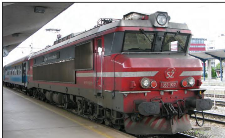
The SŽ series 363 is a class of 3 kV DC electric locos operated by Slovenian Railways & built by the French manufacturer Alstom in 1975-1977. They have a Co-Co wheel configuration & haul both passenger and freight trains. Image taken in 2008 by Ross Verdich
