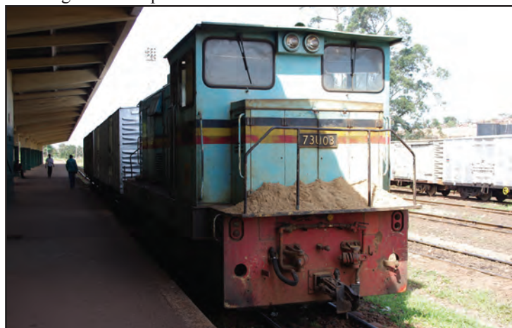
Ugandan Railways diesel locomotive 73U03 standing in Kampala station. Neville could only photograph this engine under the awning. Note the sand on the buffer beam, presumably the sanders didn't work.
