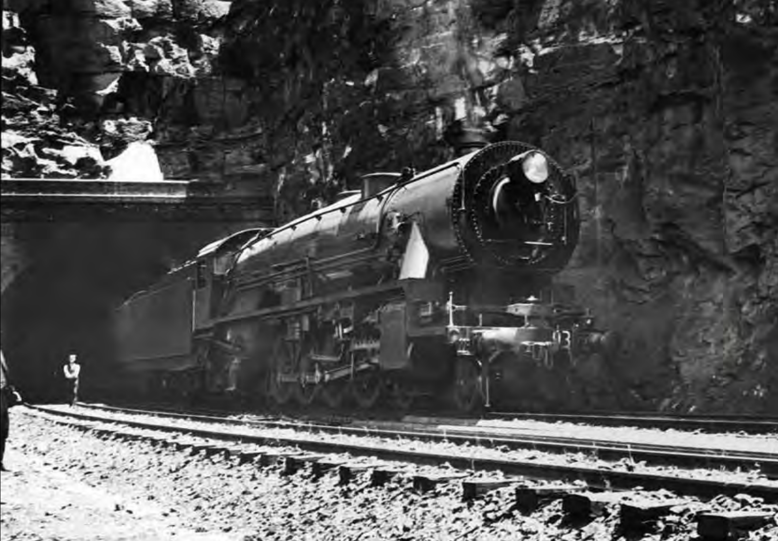
Then new 4-8-2 'Mountain' locomotive 5703 exits Glenbrook Tunnel with an Up Goods on 30 October 1929.
