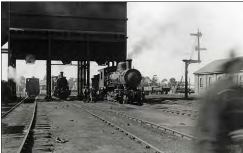
An I Class and a T Class, plus J485 in Loco at Penrith 13 February 1909. Penrith at this time was still supplying bank engines for the steep climb through the notorious single line tunnel. Note the Penrith West Box Down Distant signal on the back of the Station Box Up Home signal—a fairly common practice of the day.
