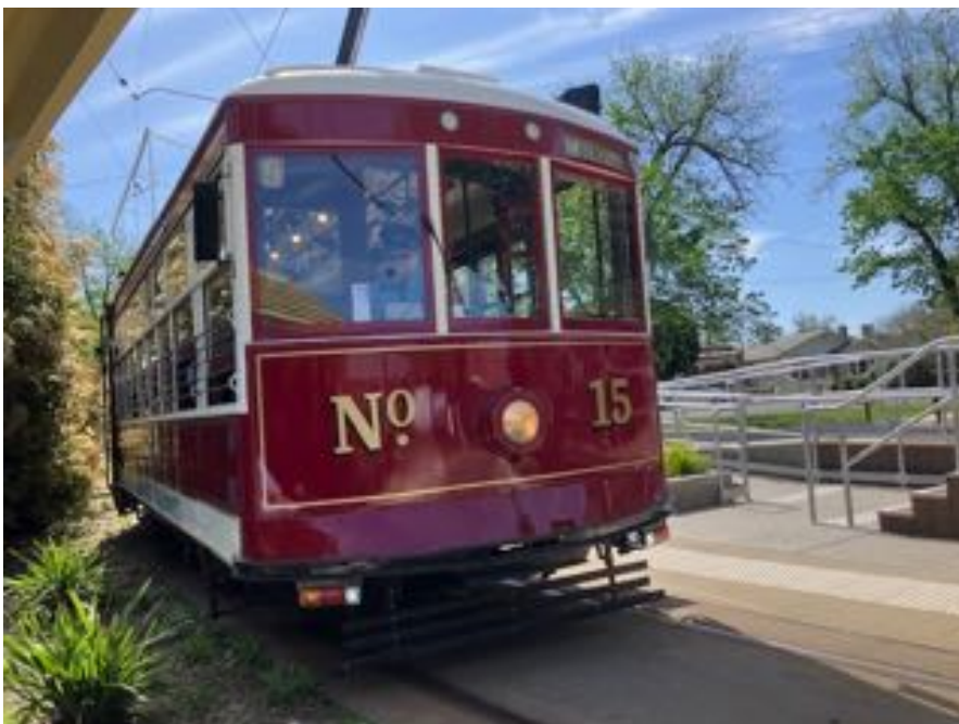
No 15 This Birney tram was built in 1924 by J.G. Brill and Co. of Philadelphia in the USA for the Melbourne Electric Supply Company, who were the operators of Geelong Tramways. The tram was flat-packed and shipped from the USA in crates and then assembled in Geelong where it operated as Tram No. 15. Image John Ruddock 2024
