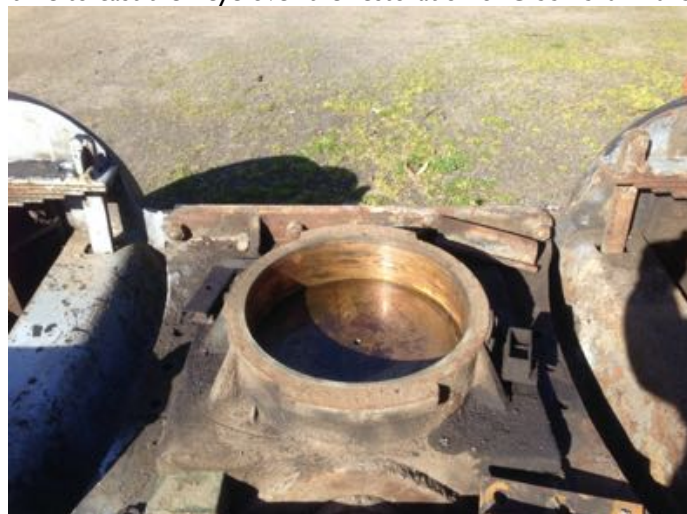
Pivot bearing on front Engine Unit Queenscliff 20130819 GWa Pic
